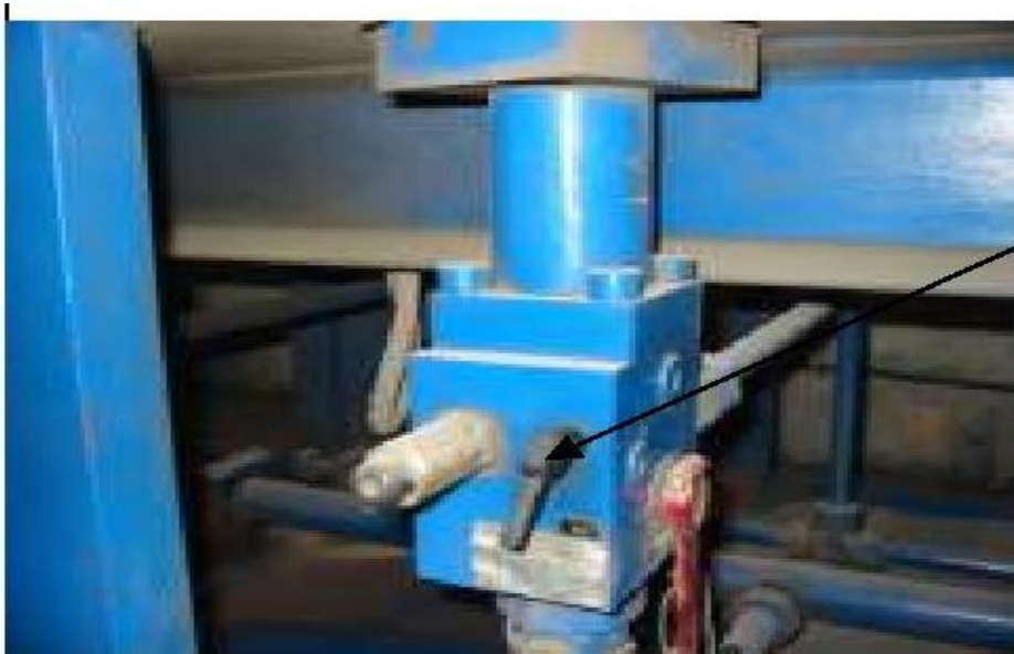
FIGURE- 3: ARROW IN THE PICTURE IS SHOWING DRAIN VALVE
