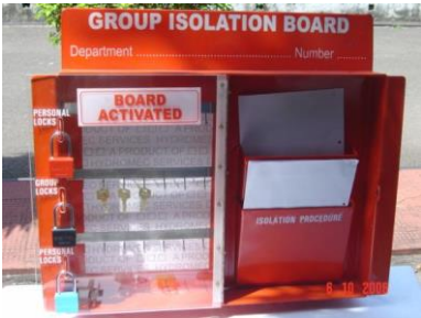
Activated Group Isolation Box with Personal Locks of Employee & Contractor and Group Isolation Lock
